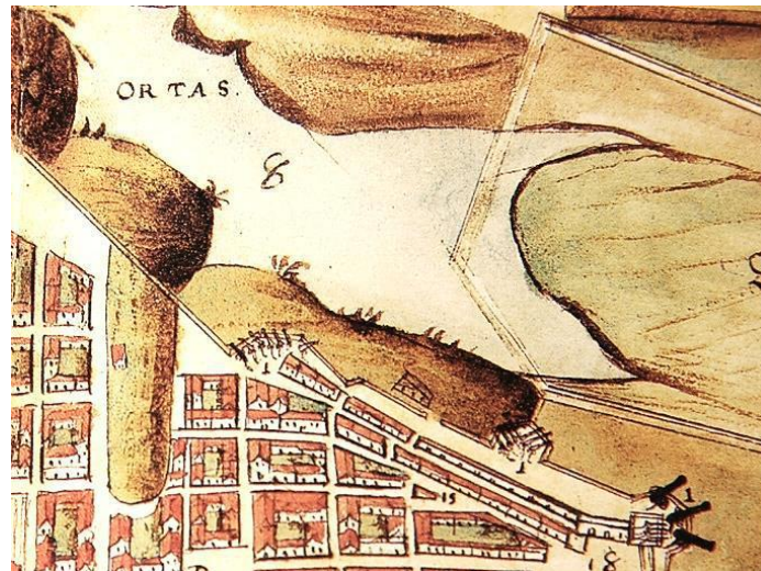
Image 47: Detail from map by Alber naz showing under number 8 the moat that the Dutch had created by making a dike that restrained the water. Note also the bulwarks, marked number 1, these were made of earth according to the legend of the map (Alber naz ca 1625).
